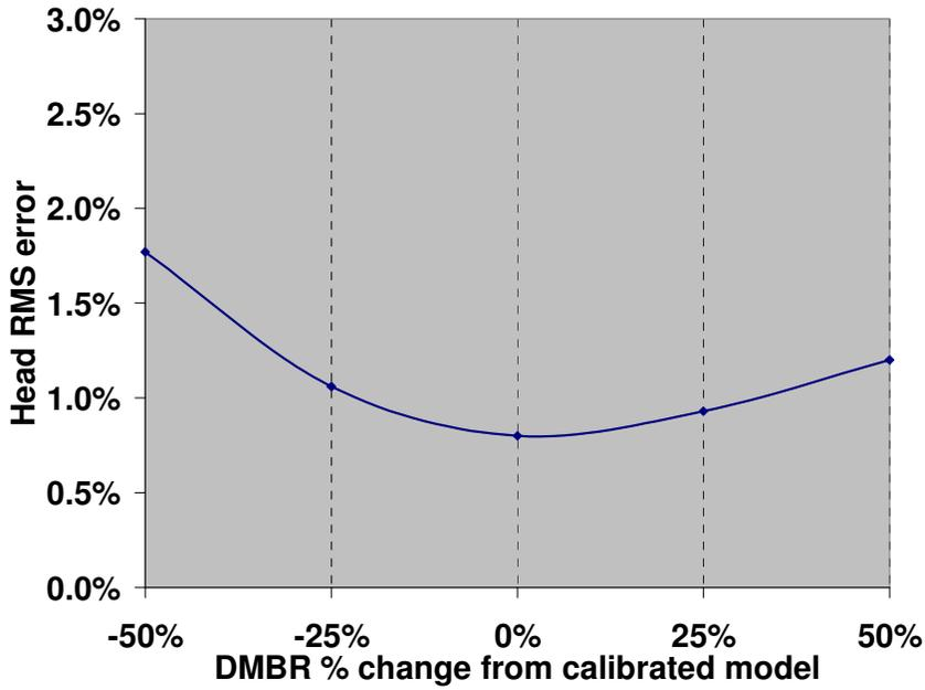
Figure 11: Head calibration sensitivity to K.
